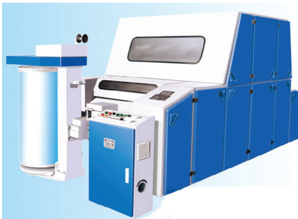
HIGH-SPEED CARDING MACHINE Model: FA206B
